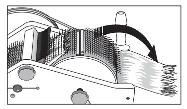
Pull the batt down over the back beam to remove it cleanly from the drum.
