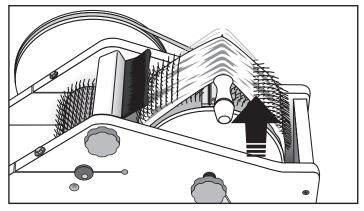
Part the batt with the doffer, taking care the doffer runs in the groove in the doffer strip.
