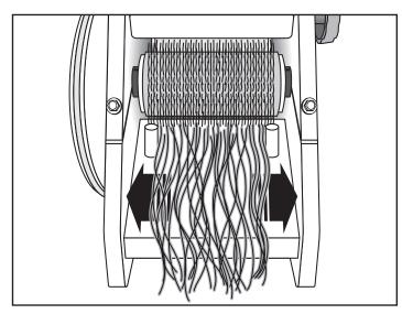
**Prepared fibre** - Peel sliver into strips, stretch to lengthen and spread it out sideways. Place on the feed-in tray and turn handle clockwise. Allow the fibres to feed-in, don't hold them back with your hand.
