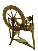
1981 - Two speed flyer with click-fit flyer bearings allow the bobbins to be changed without turning the maid upright. Tension knob is located on the front of
