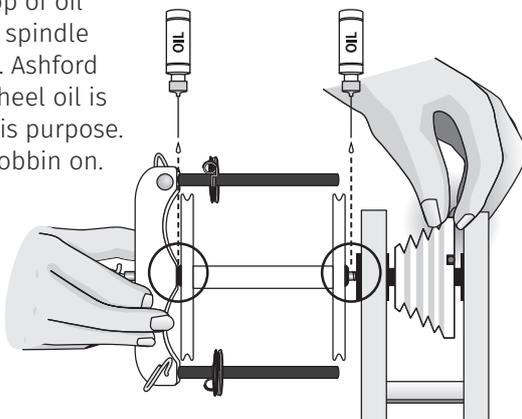
2. Screw the flyer spindle into the top shaft. Hold the flyer whorl with one hand and rotate the flyer clockwise with the other. Take care not to force or overtighten the flyer.
