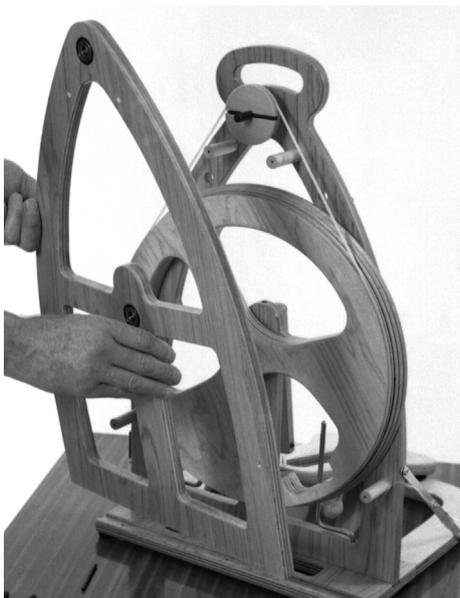
6. Carefully remove the E-Clip from the front of the flyer shaft and slide the shaft out. Carefully remove the E-Clip from in front of the pulley and slide the pulley off the shaft. Tap the tension pin out of the original flyer shaft and tap it into the new flyer shaft. Slide the pulley onto the new flyer shaft until the groove engages the tension pin. Then secure with an E-Clip. Fit the new shaft into the frame and secure with an E-Clip.
