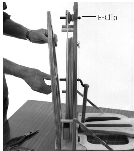
7. Place the drive belt around the wheel and pulley. Then replace the back frame into position carefully sliding the flyer and crank back through the ball bearings. **Note:** Take care not to push the ball bearings out of the plastic bearing housings.
