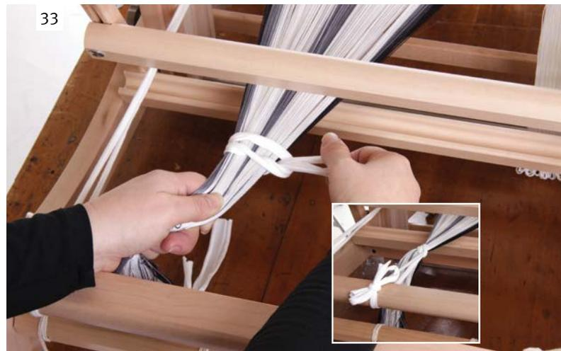
33 Take the warp through the castle to the left of the heddles. Tie the warp threads with a piece of scrap yarn using a larks head knot. Secure the scrap yarn to the front beam. Remove the tie from the end of the warp and cut the loops.
