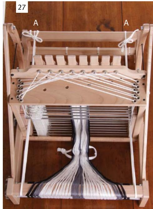
27 Attach 'helping hands' (stretchy cord included in the raddle kit) to the loom. On each side go from the front beam, through the castle, around the back beam, back through the castle and tie at the front beam (see A).
