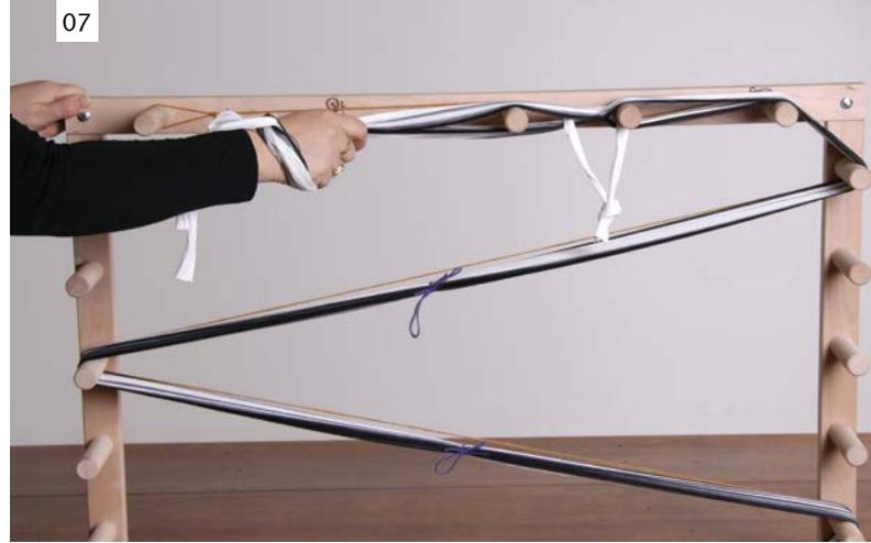
To remove the warp begin at the start peg. Take your hand through the loop and reach for the warp pulling it back through the loop. Put your hand through the new loop and continue chaining until you reach peg Y.
