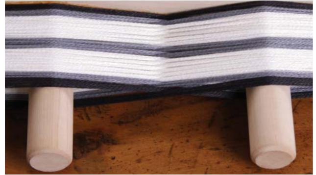
The second cross between pegs C and D is the raddle or counting cross. As the Ashford raddle has half inch (13mm) spacings and this project has a sett of 20 dpi we will make the raddle cross after each group of 10 threads.
