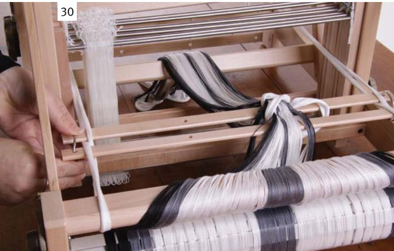
30 Secure both ends of the cross sticks with the metal rings.
