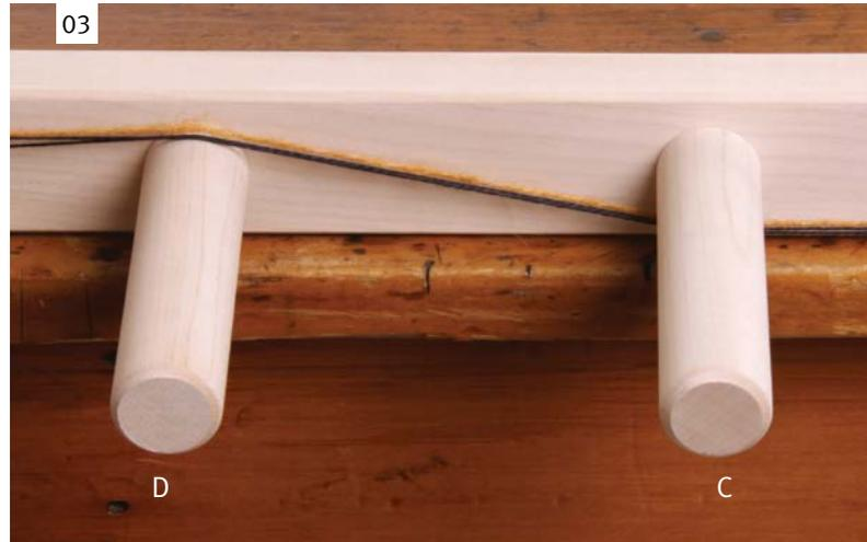
Take the yarn under C, over D and around the end peg. As the raddle cross is in groups of 10, return over D and under C for 10 threads (5 return trips). The eleventh thread will go over C, under D, around the end peg, back under D and over C. Now follow the warp colour order on the previous page.
