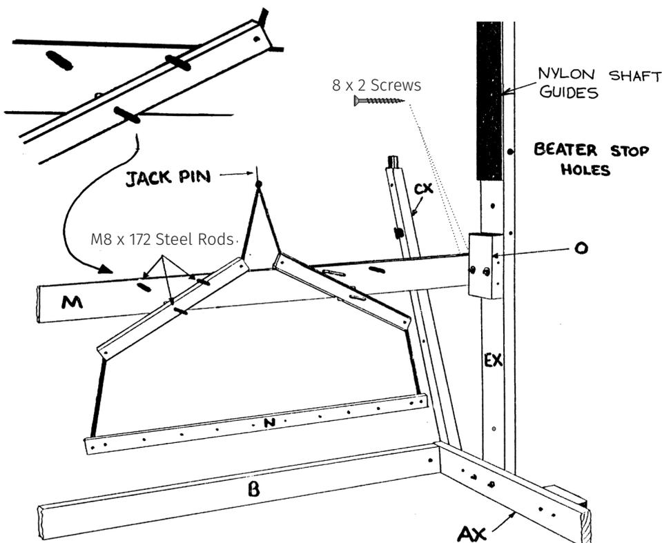
4. Secure one rail **M** to blocks **O** using two 8 x 2 Screws at each end. Note the position of the holes for the steel rods **x**.
