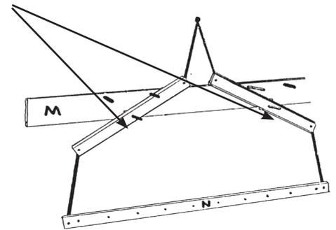
7. Locate the second rail **M** onto the steel rods and secure to blocks **O** using two 8 x 2 Screws at each end.
