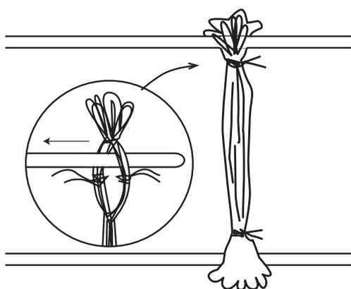
23. Wipe the stainless steel bars with a clean cloth to remove any protective grease. Your Ashford 8 Shaft Jack Loom has been supplied with Texsolv Heddles. Each bundle contains 100 heddles which enable you to use 100 per shaft.
