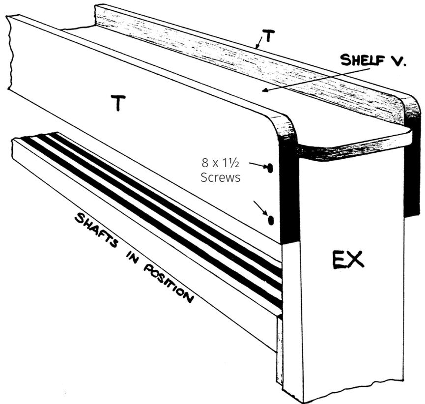
27. Locate the front and back beams Y onto the tenons of uprights C, CX and D, DX. The beams are easily removable to allow access to the shafts when warping.
