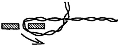
Then take the long end of the cord through the small hole in the warp roller and out the large hole. Then push a Texsolv peg through the cord. The peg pulls down flat into the large hole.
