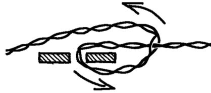
Then take the long end of the cord through the small hole in the warp roller and out the large hole. Then push a texsolv peg through the cord. The peg pulls down flat into the large hole.
