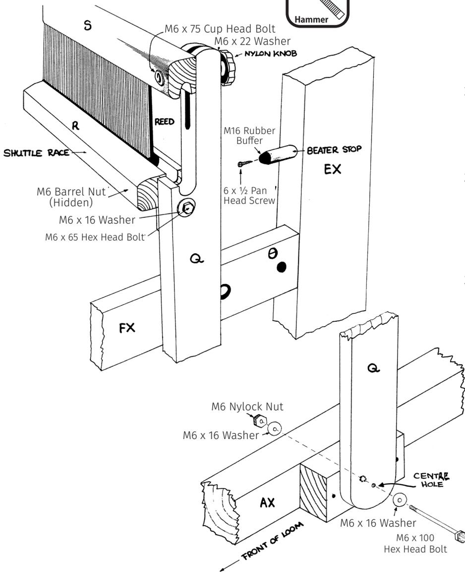
28. Tap the beater stops into the castle sides E and EX. Note the lead holes for the screws face out. Use wood glue if necessary. They should project approx. 70mm (2¾"). Then attach the M16 Rubber Buffer to the stops with 6 x ½ Pan Head Screws.
